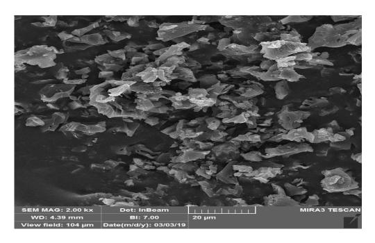
Figure 4. FESEM image of the pine bark biochar after diclofenac adsorption
