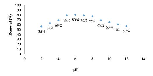
Figure 5. Effect of pH on diclofenac removal efficiency (C=50 mg/L; adsorbent dose= 0.8 gr; time= 15 min; T=25 °C)
