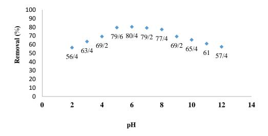
Figure 5. Effect of pH on diclofenac removal efficiency (C=50 mg/L; adsorbent dose= 0.8 gr; time= 15 min;  $T=25 \text{ }^{\circ}C$ )
