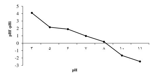
Figure 2. The point of zero charge determine in the pine bark biochar
