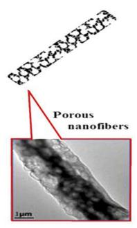
Scheme 1. Electrospun nanofibers with high porosity and small pore size (24)
